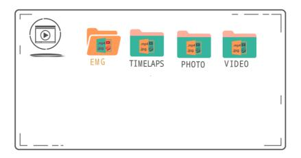
**Note**: There are four folders in it, among which EMG and TIMELAPS are the system built-in folders, PHOTO is the photo folder, and VIDEO is the video folder. The operation method is the same after entering the PHOTO and VIDEO sub-files.
