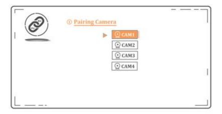
**Note:** Code pairing is required as follows. Use the up and down keys to select the Pairing Camera option, and then press the enter key to enter the code pairing sub-menu interface, the interface is as follows:
